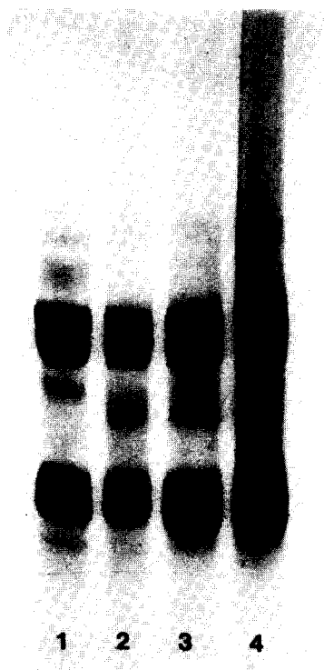
Fig. 3. SDS-polyacrylamide gel electrophoresis pattern of apricot kernel proteins in 0.125M tris-borate buffer of pH 7.1 containing 0.1% SDS. 1,2: flour and protein isolates extracted at pH 7.7. 3,4: flour and protein isolates extracted at pH 12.0.
